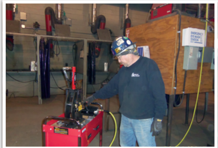
Local 424 Apprentice Coordinator John Jones utilizing the new hydraulic bender to test weld plates.
